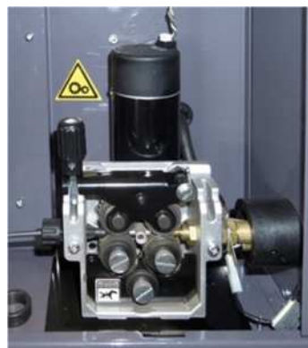
Trainafilo a 4 rulli 4-roller wire feeder
