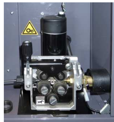
Trainafile a 4 rulli 4-roller wire feeder
